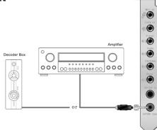
Plug the optical TOSLINK adaptor into the S/PDIF-Out combo connector. Then, connect your decoder's S/PDIF in port to the optical adaptor with the TOSLINK optical cable
